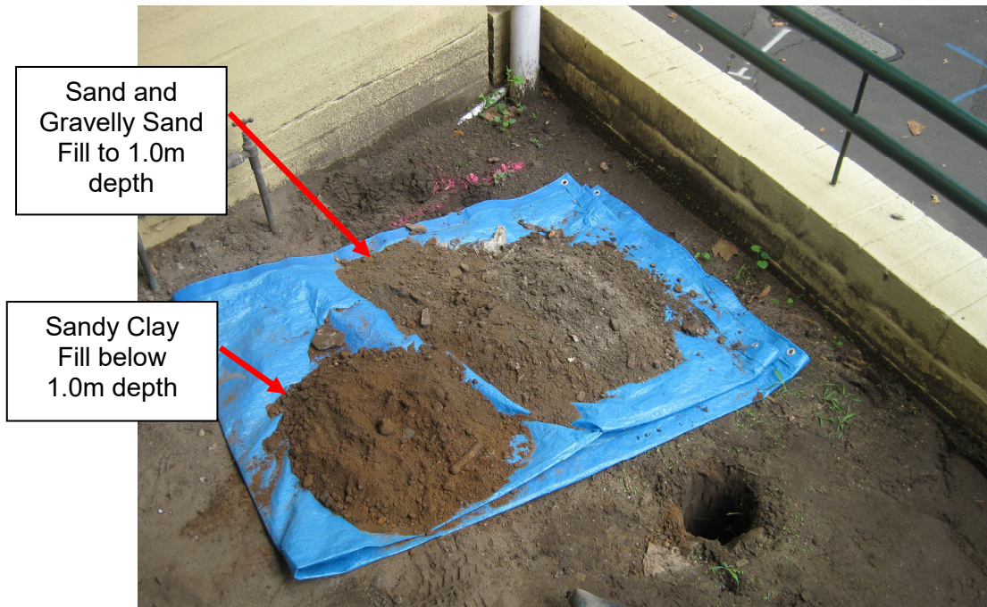
Photograph 14 – View of drilling spoil obtained from Borehole BH7.
